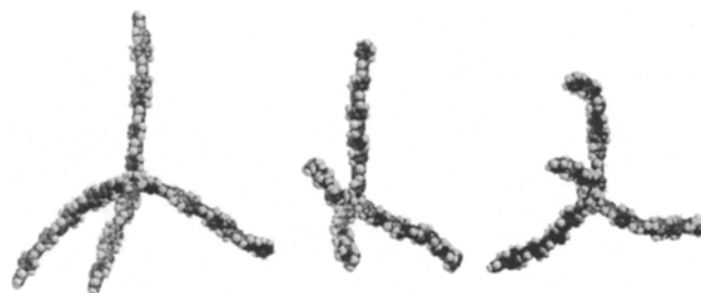
Fig. 2 Shapes of the adamantane-based multipodes with long arms at various temperatures (300 K, 500 K, 700 K)
